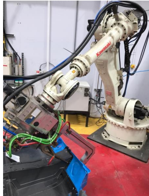
Robotic joining of a carbon fibre battery housing to steel car body components
